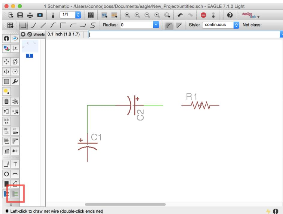
**Figure 8: Components With Nets Being Placed**
