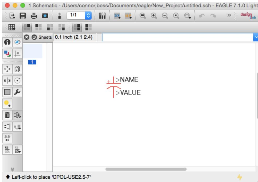
**Figure 7: Component Placed in Schematic Workspace**
