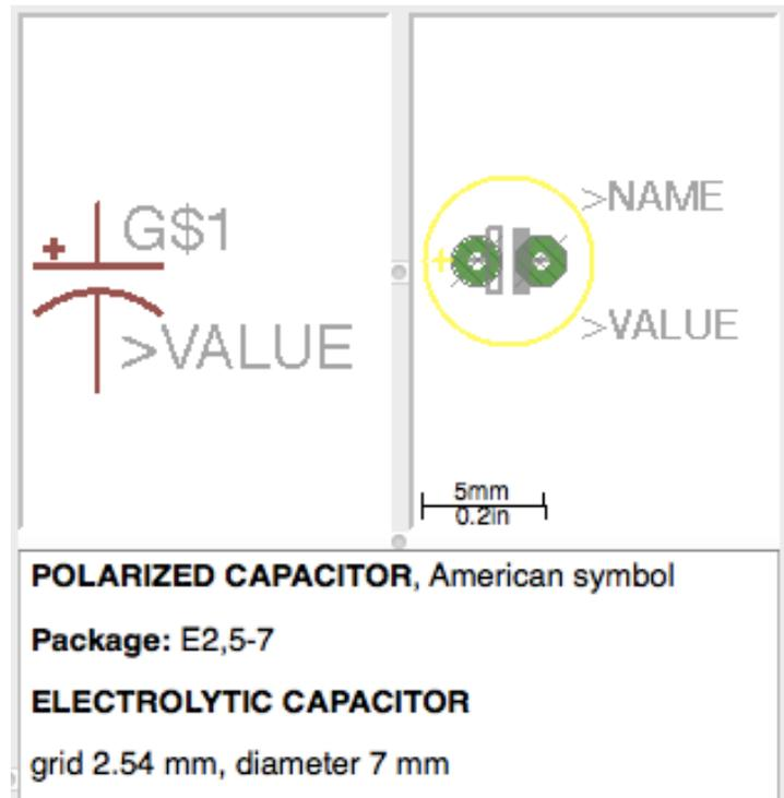
**Figure 6: Schematic and Printed Circuit Board Symbols**
