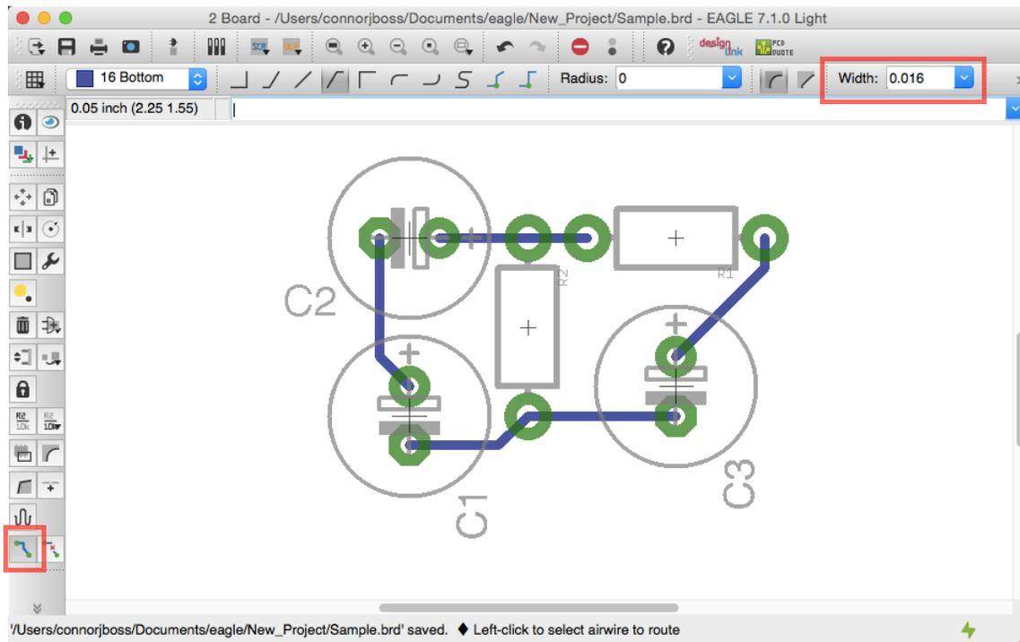
**Figure 11: Fully Routed Printed Circuit Board**
