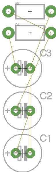
Figure 10: Board File Generated From Schematic
